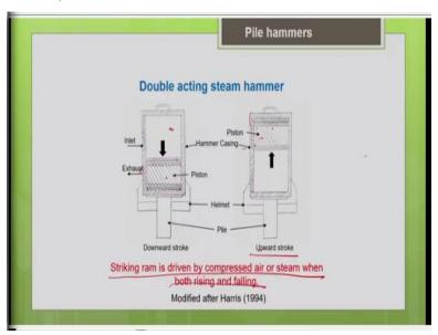
So, the striking ram is driven by compressed air or steam, when both rising and falling.
