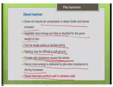
The main advantage is it does not require a separate air compressor or steam boiler and hence very compact. And the available input energy per blow is doubled for the given weight of ram, how it is double? Because of the explosive energy we get additional energy for driving, so it can be also either single acting or double acting. So, as I told you in a soft ground, the initiation of the process is difficult.
