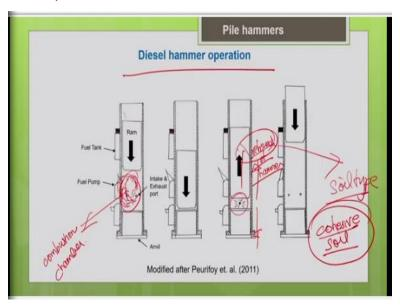
So, we have completed the double acting stream hammer, now let us move on to diesel hammer. So, basically this diesel hammer is a self-contained unit, that means everything is contained within a single assembly, I do not need a separate accessory a steam boiler or air compressor as we need it for the steam hammers. Everything is contained within a single unit you can see, so what will be the advantage?
