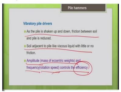
So, as your pile is shaken up and down, consider the friction between the soil and the pile will be reduced, so that will facilitate easy penetration of a pile into the ground. Because of the vibration, the soil adjacent to the pile will behave like a liquid, with little or no friction which facilitates penetration of the pile into the ground. Your amplitude of the vibration will depend upon your mass of the weights, eccentric weights inside your vibrator.
