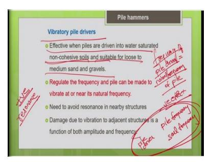
So, for what type of soil this is more preferable, this is more preferable for non-cohesive soil because that will respond easily to the vibration when compared to cohesive soil. So, this is particularly for water saturated soil, this is the right choice. So, this is effective in the piles are driven into water saturated non-cohesive soil and suitable for loose to medium sand and gravel because these kinds of soil will respond well to the vibration.
