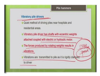
So, the last type of pile which we are going to discuss is about the vibratory pile driver. So, for whatever we discuss on impact hammers, which results in lot of noise production as we discussed earlier. And this method may not be feasible, if you are going to do a pile driving operation in a residential colony or near schools or hospitals where we need silent pile driving method.
