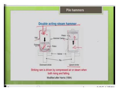
So, basically what to do here is, so this is a setup of the double acting steam hammer, you can see two cylinders one is the upper cylinder, other one is a lowest cylinder. Now in the upward stroke what you do is, you supply air into the lower cylinder. So, when you supply into this, this is a lowest cylinder, when you supply air into the lower cylinder, the hammer which was earlier in the lower cylinder will be pushed up into the upper cylinder.
