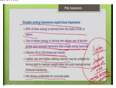
So, another important thing we need to know with respect to double acting hammer is in this most of the blow energy is the derived from the steam energy. Both for the upward stroke as well as for
