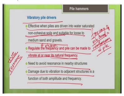
You regulate the frequency and the pile can be made to vibrate at or near it is natural frequency, you regulate the frequency of the pile driver and the pile can be made to vibrate at or near it is natural frequency. So, this will result in positive impact of resonance, which will make your pile driving operation easier. Another important thing is you need to avoid the resonance in the nearby structures, make sure that the frequency of the structure should not coincide with your pile driving.
